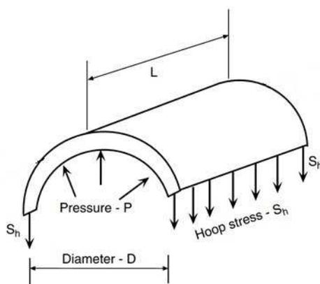
Considering the one-half section of the casing and balancing the forces acting on the two rectangular areas  $L \times t$ , against the internal pressure on the projected area  $D \times L$  which is therefore,
