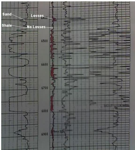
**Figure 1—Log section showing indications of “normal” losses of drilling mud in sands.**
